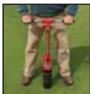
1. Place HIO Hole Cutter in desired cup location.
