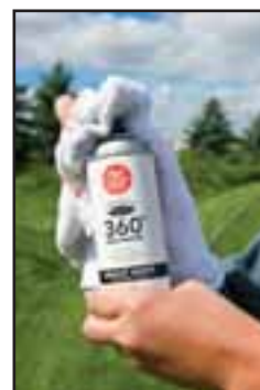
5. Place rag over nozzle and press to clear excess paint from nozzle after each hole is painted.
