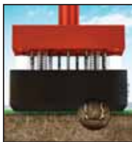
Spikes retracted, leaving seed in holes.
