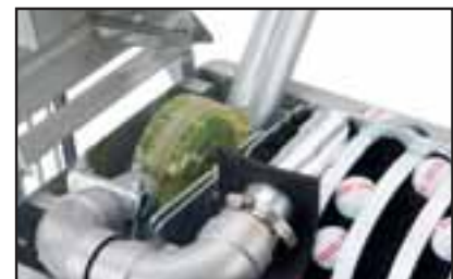
After washing the composite loader wheel pushes the balls into the feeder pipe.
